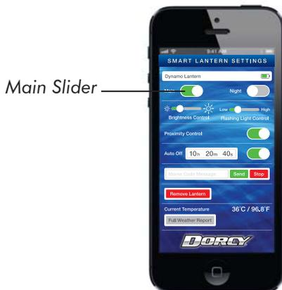
Move the MAIN slider to the right to turn on the lantern. (Note that when the MAIN light is on the night light cannot function at the same time).
