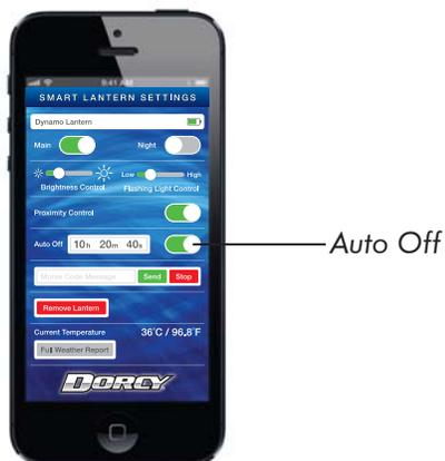
You can set the lantern on a timer to automatically shut off at a certain time. Make sure the slider is showing green and enter the time in which you want the lantern to shut off.
