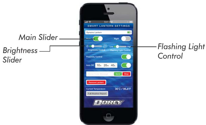
To control the brightness of the MAIN lantern use the slider on the Brightness control to go from a softer light to a brighter light.
