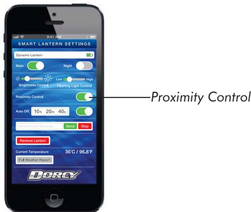
The proximity control feature can be used for when the device running the App is more than - - feet away the lantern will shut off. Then when the device is back within the range of the lantern, the light will come back on to the original setting that it was left at.
