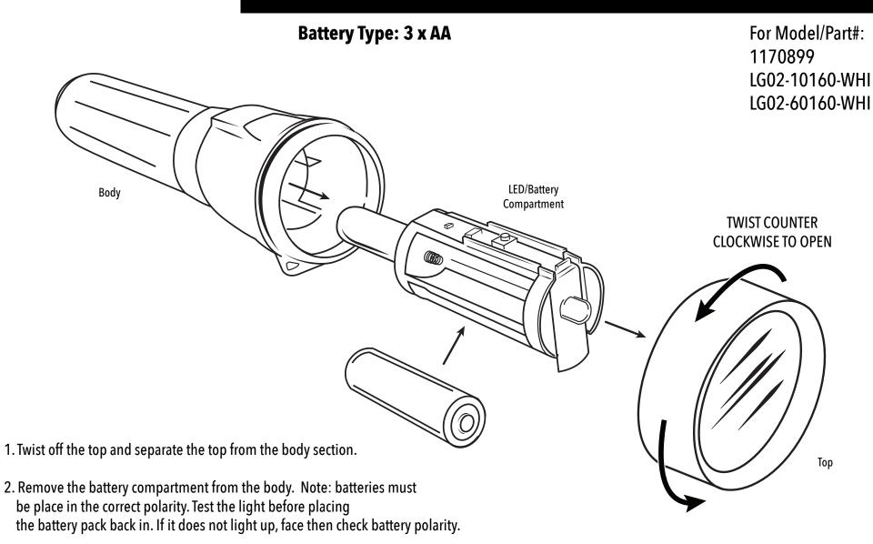
3. After replacing batteries, install the battery pack with the circuit side lined up with the on/off button on the body. Slide in and twist on the top.
