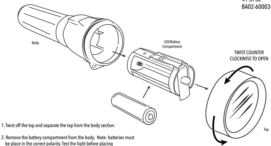
3. After replacing batteries, install the battery pack with the circuit side lined up with the on/off button on the body. Slide in and twist on the top.
