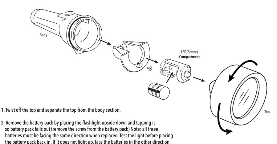
3. After replacing batteries, install the battery pack with the circuit side lined up with the on/off button on the body. Slide in and twist on the top.
